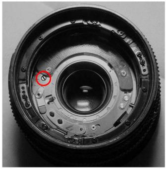
The trimmer is accessible through a hole, the side picture shows a PS lens with brand name plate and frontal optical assembly removed; the red circle marks the trimmer screw.
